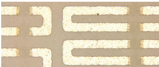
Platinum film links cut with short-pulse laser.
